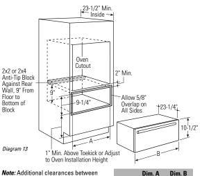
**Note:** Additional clearances between cutouts may be required. Check to be sure that oven supports above the Warming Drawer location does not obstruct the required interior 23-1/2" depth and 9-1/4" height.
