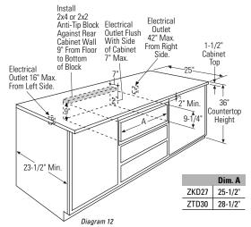
$\it \textit{Note}$ : When installing the Warming Drawer below a cooktop, allow a 2" min. clearance between the bottom of the cooktop burner box to top of cutout.
