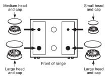
B. Make sure the slot in the burner head is positioned over the electrode (on some models).
