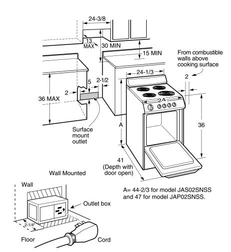
Recommended acceptable electrical outlet area. Orient the electrical receptacle so the length is parallel to the floor.
