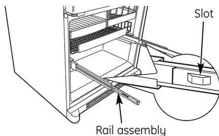
**C** Insert the hooks at the back of the drawer railings into the slots on the rail assemblies.
