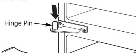
**B** Securely tape the door shut with masking tape or have a second person support the door.
