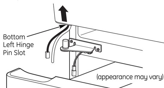
**D** On left-hand doors, pass the wires and water line through the center hinge pin. Then connect the water line and 4-pin connector.
