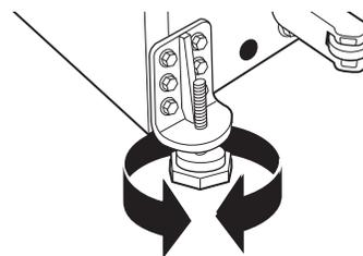
If the doors remain uneven, turn the adjustable pin to raise, or lower, the left door to match the right door. Use a 1/4" Allen wrench to turn the pin.
