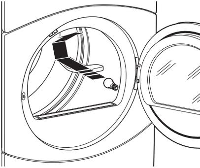
Before replacing the light bulb, be sure to unplug the dryer power cord or disconnect the dryer at the household distribution panel by removing the fuse or switching off the circuit breaker. Reach above dryer opening from inside the drum. Remove the bulb and replace with the same size bulb.
