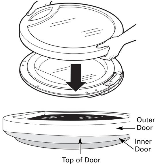
After reversing door, there will be a mismatch between the outer door and the inner door.
