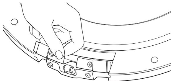
Secure the hinge cover with the 2 tapping screws (#8).
