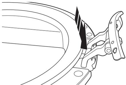
Push the hinge assembly into place until the hinge holes align with the door holes.
