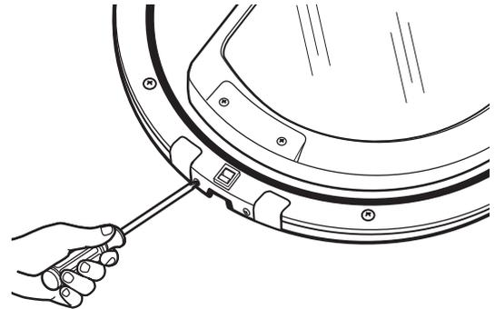
Remove the window retainer and set it aside. The window retainer is located on the side opposite the hinge assembly and underneath the plastic cover.
