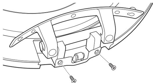
Hold the door on its side with one hand and fasten the remaining 2 screws as shown.
