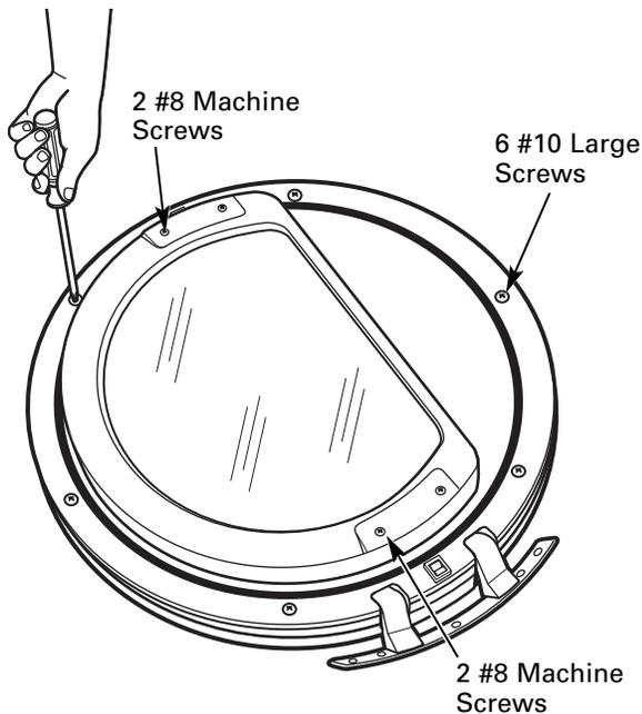
With the screws removed, turn the door over and separate the silver cover part of the door from the door frame and set aside.
