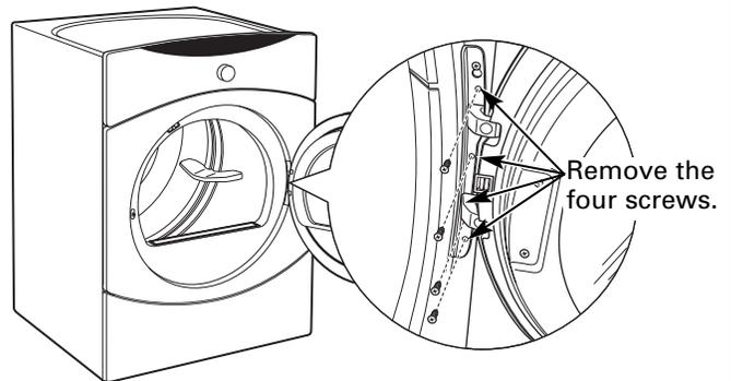
Loosen the top screw as shown. Unhook the door by lifting and pulling as shown by the arrows.
