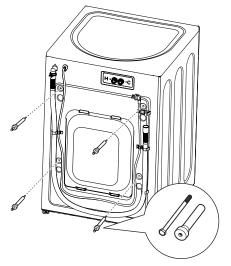
**NOTE:** Failure to remove the shipping braces can cause the washer to become severely unbalanced.
