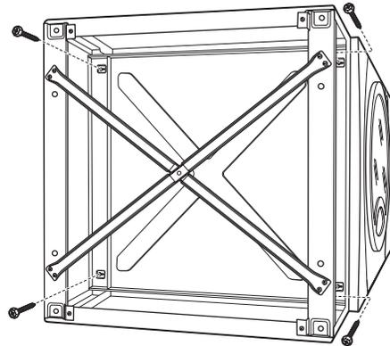
**C** Slide the pedestal toward the unit, until it is aligned front to back. Use an 8 mm socket wrench to securely tighten the screws.
