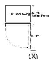
Allow 25" minimum clearance for a full 130° door swing. Allow 15" for pan removal. for a 90° door swing, allow 5" minimum clearance for professional models. If the 90° doorstop position is used, pan access is maintained but pan removal is restricted.
