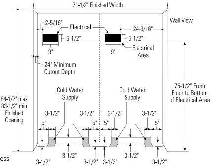
If you are installing two units, side by side, the installation space must be 71-1/2" wide. Additional cutout width may be required when side panels are used. Add side panel thickness to the finished cutout to calculate rough-in width.
