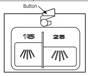
To open the wash cover, press the button and the cover will flip back.
