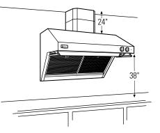
**9 ft. ceilings:** When the hood is installed 38" above the cooking surface, order two 12" duct cover accessories.
