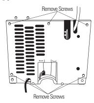
• Remove screws holding the rear cover. Retain screws. Carefully pull rear cover away from drain tube.
