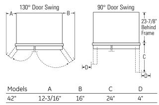
Allow minimum clearances for Freezer door (Dimension A) and Fresh Food door (Dimension B) for a full 130° door swing and to allow for drawer removal.
