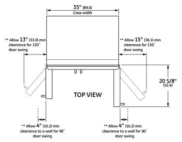
\*\* These refrigerators are equipped with a 2-position door stop. The factory-set 130° door swing can be adjusted to 90° if clearances to adjacent cabinets or walls is restricted. Allow full 130° door swings for pan removal. If the 90° door stop position is used, pan access is maintained, but pan removal is restricted.
