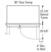
Allow minimum clearances for freezer door and fresh food door for a full 130° door swing and to allow for pan removal.
