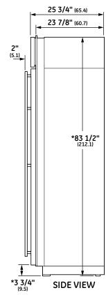
\* Shipping height. Use leveling legs and wheels for maximum 1" height adjustment from shipping height.
