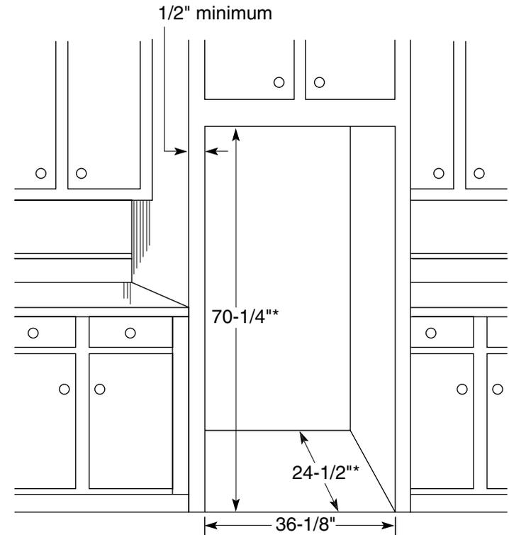
\*The rough-in dimension of 70-1/4" is minimum and is measured from the finished floor to top of opening (or the underside of the overhead cabinets). For Models with Trim Kit: If frameless style cabinets are planned for above the refrigerator, you may need to consider adding a maximum of 1/4" (70-1/2") to height of opening to allow additional clearance between cabinet doors and top of refrigerator trim when cabinet doors are in open position.
