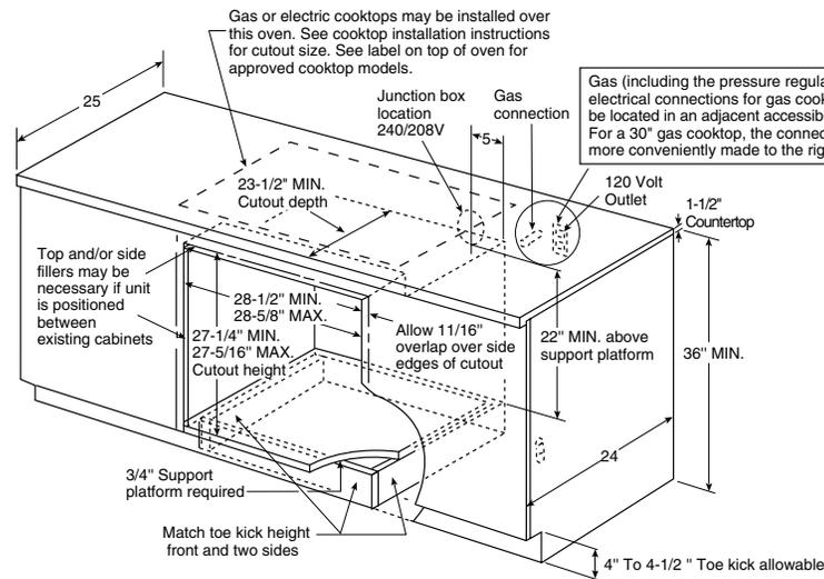
**Note:** 36" ribbon cooktops are approved for use over GE 30" single wall ovens only. 30" ribbon cooktops are approved for use over GE 30" and GE 27" single wall ovens. Refer to cooktop and wall oven installation information packed with products for current dimensional data.
