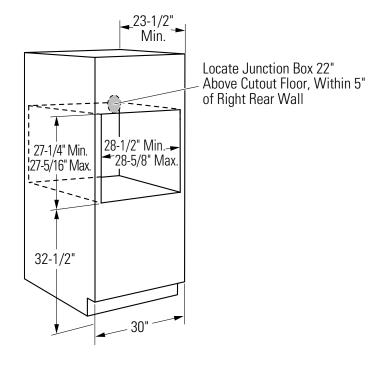
The solid bottom or runners must be level with the bottom of the cutout, or the bottom trim may not install correctly and could interfere with the door opening. If the cabinet does not have a solid bottom, two braces or runners must be installed level with the bottom of the cutout to support the weight of the oven. The runners and braces must support 150 lbs. (68 kg).
