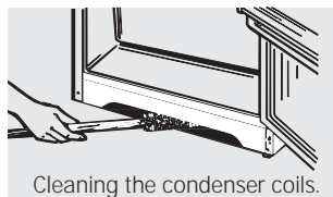
Cleaning the condenser coils.
