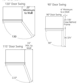
Allow 25" minimum clearance for a full 130° door swing. Allow 15" for pan removal.
