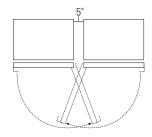
Clearances for two products installed side-by-side with right and left side hinges together
