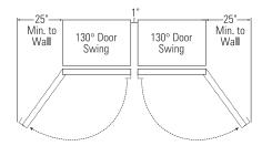
Clearances for Multiple Single Door Installations In a side-by-side installation of a left and right door swing product, a 1" clearance between the units is required. Order ZUGSS2 Stainless Steel Unified Grille Panel Kit or ZUG2 Custom Panel Unified Grille Panel Kit for one continuous grille panel.
