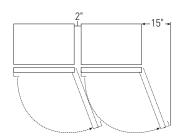
Clearances for two products installed side-by-side with the same (left or right) door swing
