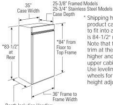
\* Shipping height. The product can be adjusted to fit into a cutout that is 84-1/2" max. height. Note that the top case trim at the front is 1/2" higher and will overlap upper cabinetry or soffit. Use leveling legs and wheels for a maximum 1" height adjustment.
