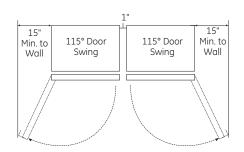
Clearances for Multiple Single Door Installations In a side-by-side installation of a left and right door swing product, a 1" clearance between the units is required. Order ZUG2 Unified Grille Panel Kit for one continuous grille panel.
