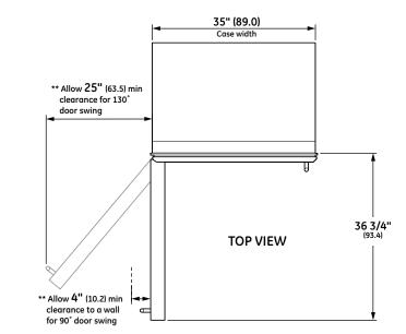
\*\*These units are equipped with a 2-position door stop. The factory set 130° door swing can be adjusted to 90° if clearance to adjacent cabinets or walls is restricted. Allow 15" minimum clearance to wall for pan removal. If the 90° door stop position is used, pan access is maintained but pan removal is restricted.
