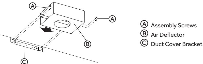
2. Measure from the bottom of the air deflector to the bottom of the hood exhaust outlet.
