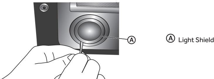
3. Gently pull the burned out bulb from the socket.
