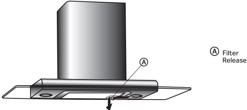
2. Wash the metal filter, as needed, either in the dishwasher or with a solution of hot water and dish detergent.
