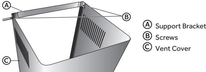
2. Attach support bracket to wall flush to the ceiling using two - 5 x 45 mm screws.
