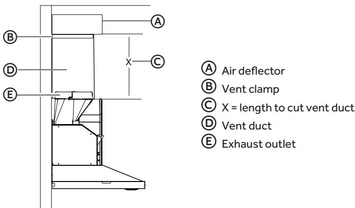
3. Cut the duct to the measured size (X).
