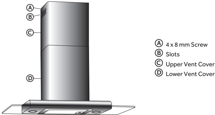
2. Using two screws (provided) fasten the bottom of the duct to the hood.
