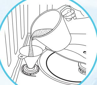
4. Slowly fill the container with the dishwasher water softener salt. The salt container holds approximately 4½ cups (1.0 kg) of salt. As it is being filled, some water will run out.
