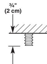
6. Screw the nuts on the hanger bolts, but do not tighten.
