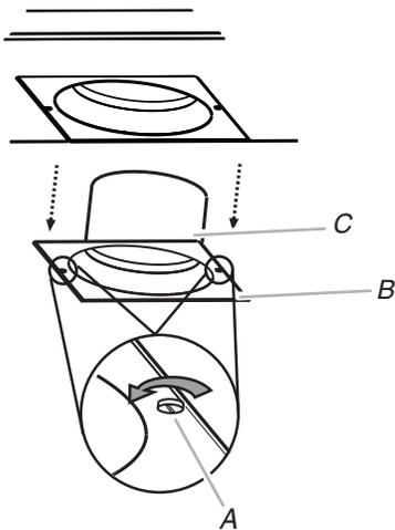
A. Grease filter release screw
