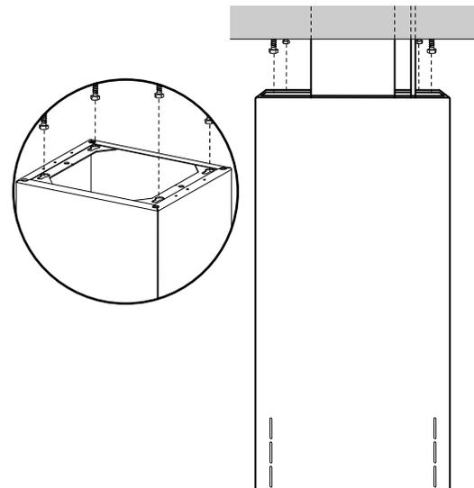
2. Using the ½" (13 mm) special tool (supplied) or a ½" (13 mm) socket and driver with 24" of extensions, tighten the nuts to fasten the upper chimney cover section to the ceiling.
