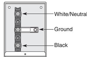
This unit is supplied with an electrical junction box on a 48" long, 1/2" (1.3 cm) I.D. flexible conduit. The junction box is designed to be attached to a solid mounting surface in the area below the cooktop. Connect all supply wires to the power block with approved connectors. Bare wires can be attached using the supplied bare wire adapter lugs. All connections should be torqued to 20 in-lb.
