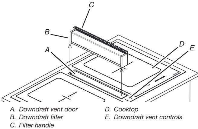
The downdraft vent removes cooking vapors, odors, and smoke from the cooktop area. The downdraft vent consists of a vent filter, vent ducting, and a vent fan.
