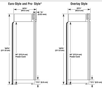
"When leveling legs are fully extended to 1<sup>1</sup>/4" (3.2 cm) below rollers, add 1<sup>1</sup>/4" (2.9 cm) to the height dimensions.
