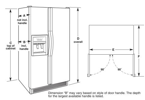
Dimensions "C" and "D" include the leveling legs extended to the minimum height of  $\frac{1}{2}$ " (6.35 mm) below the refrigerator. When leveling legs are fully extended to 1" (2.54 cm), add  $\frac{3}{2}$ " (19.05 mm).
