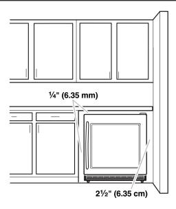
To ensure proper ventilation for your beverage center, allow for a  $\frac{1}{4}$ " (6.35 mm) space on each side and at the top. When installing your beverage center next to a fixed wall, leave  $2\frac{1}{2}$ " (6.35 cm) minimum clearance on each side to allow for the door to swing open.
