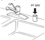
that the drain hose either be looped up and securely fastened to the underside of the counter, or be connected to an air gap.
