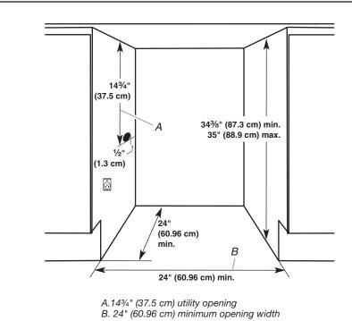
Height dimensions are shown with the leveling legs extended to the minimum height. NOTE: When leveling legs are fully extended, add 5%" (15 mm) to the height dimensions.
