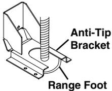
**Making sure the anti-tip bracket is installed:**
