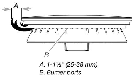
**Burner ports:** Check burner flames occasionally for proper size and shape as shown above. A good flame is blue in color, not yellow. Keep this area free of soil and do not allow spills, food, cleaning agents or any other material to enter the burner ports.
