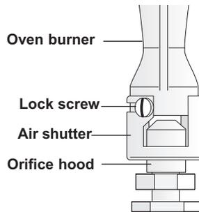
Fig. 21 - typical oven burner air shutter
