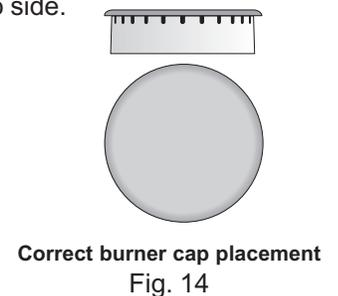
Correct burner cap placement
