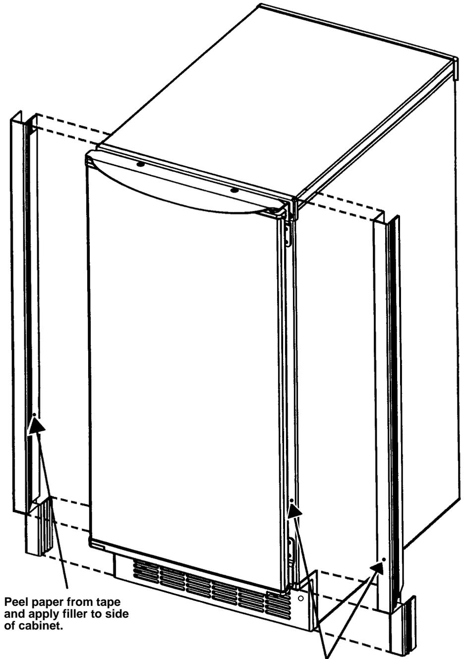
Peel paper from tape and apply filler to side of cabinet.
