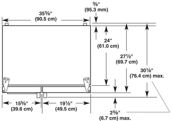
■ Height dimensions are shown with the leveling legs extended to the minimum height of 1¼" (6.35 mm) below the refrigerator.
