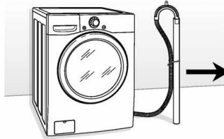
Connecting the drain line
