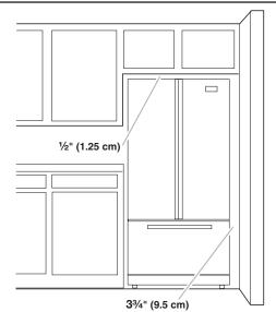
To ensure proper ventilation for your refrigerator, allow for a  $\frac{1}{2}$ " (1.25 cm) space on each side and at the top. Allow for 1" (2.54 cm) of space behind the refrigerator. If your refrigerator has an ice maker, make sure you leave some extra space at the back for the water line connections.
