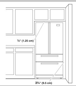
To ensure proper ventilation for your refrigerator, allow for a ½" (1.25 cm) space on each side and at the top. Allow for 1" (2.54 cm) of space behind the refrigerator. If your refrigerator has an ice maker, make sure you leave some extra space at the back for the water line connections.
