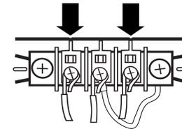
4. Tighten strain relief screws.
