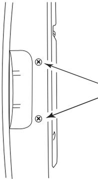
4. Remove the 6 screws to release the outer door assembly from the inner door assembly (see illustration). It is important that you remove only the 6 indicated screws.
