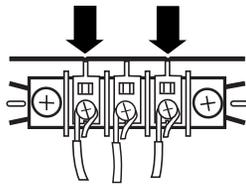
4. Tighten strain relief screw.
