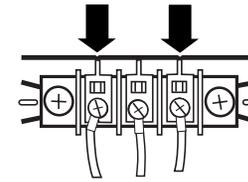
4. Tighten strain relief screws.
