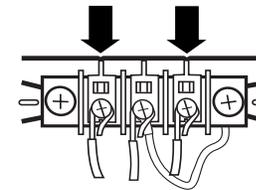
5. Tighten strain relief screw.
