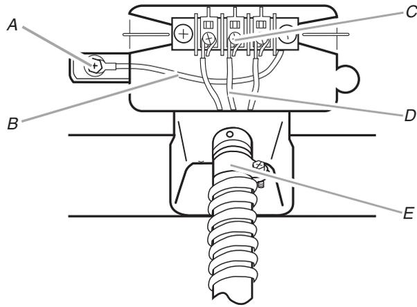
A. External ground conductor screw
