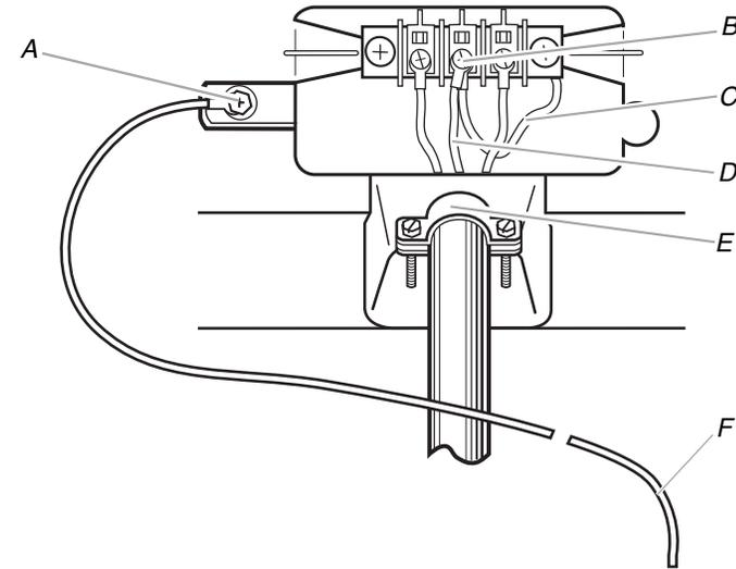
A. External ground conductor screw
