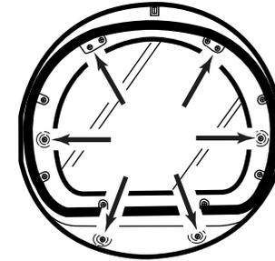
5. Lift the inner door assembly off of the outer door assembly. Unsnap the handle from the outer door assembly, move it to the other side, and snap in. Set the outer door assembly aside.
