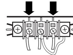
5. Tighten strain relief screws.
