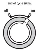
Turn the END OF CYCLE SIGNAL knob to select the desired setting (On or Off). The End of Cycle Signal produces an audible sound when the drying cycle is finished. Promptly removing clothes at the end of the cycle reduces wrinkling.
