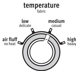
Select temperature by turning the knob to the desired position or select the Automatic Dry Cycle that has the temperature included in the cycle selections.
