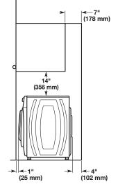
All dimensions show recommended spacing allowed, except for closet door ventilation openings which are the minimum required.
