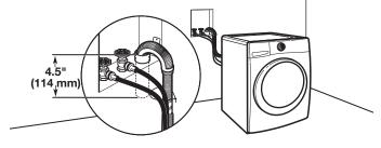
See requirements for floor standpipe drain system.
