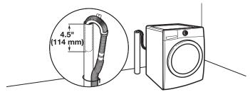
Minimum diameter for a standpipe drain: 2" (51 mm). Minimum carry-away capacity: 17 gal. (64 L) per minute. A 1/4" (6 mm) diameter to 1" (25 mm) diameter Standpipe Adapter Kit is available (Part Number 3363920). Top of standpipe must be at least 30" (762 mm) high; install no higher than 96" (2.44 m) from bottom of washer. If you have an overhead sewer and need to pump higher than 96 inches, a sump pump and associated hardware are needed. See "Alternate Parts".
