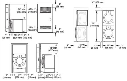
\* required spacing \*\* for venting out the side, 1" (25 mm) spacing is allowed.
