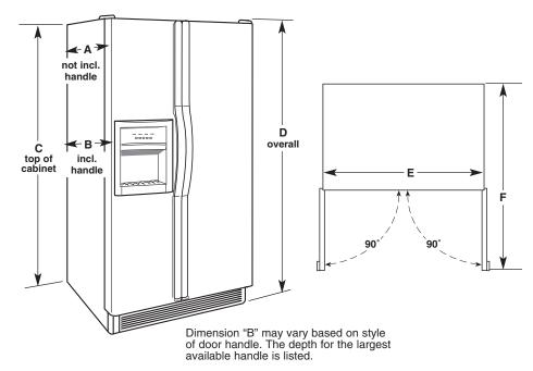
Dimensions "C" and "D" include leveling legs extended 3/4" (1.9 cm).
