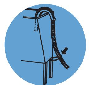
Secure the drain hose with beaded tie strap, in one of these ways:
