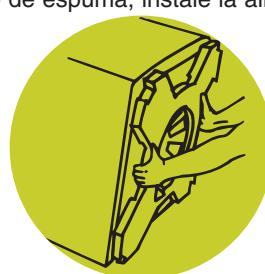
Lay washer on its back and remove foam shipping base.
