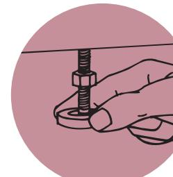
Push on the upper front panel to be sure that the washer is on the rear feet.
