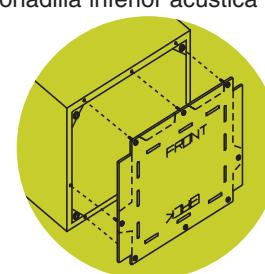
Insert lower sound pad by aligning plastic fasteners to bottom of cabinet, fold front tabs (2) into lower cabinet. See Use and Care Guide.
