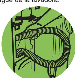
Locate the pull tie to remove drain hose from washer. Pull drain hose straight out of washer by first grabbing the pull tie.
