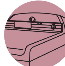
Check levelness by first placing level on the lid near the console.
