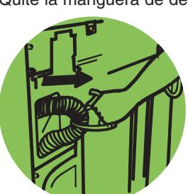
Remove drain hose from washer.
