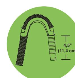
Retrieve hose form from parts bag. Feed drain hose into one end of form. Place end of form into the drain hose relief.
