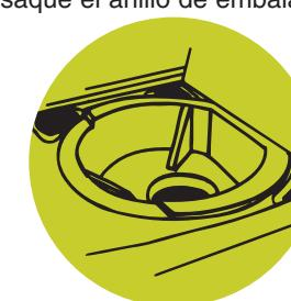
Set washer upright. Remove tape and lid label from lid. Remove foam packing ring from washer tub.
