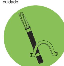
Pull drain hose straight out of washer from top of hose. Continue to pull the hose until the end emerges.
