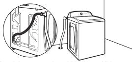
Floor drain system requires additional parts. Minimum siphon break: 28" (710 mm) from bottom of washer.
