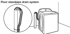
Minimum diameter for a standpipe drain: 2" (51 mm). Minimum carry-away capacity: 17 gal. (64 L) per minute. Top of standpipe must be at least 39" (990 mm) high; install no higher than 96" (2.44 m) from bottom of washer. If you must install higher than 96" (2.44 m), you will need a sump pump system.
