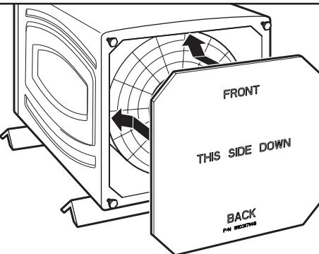
Orient the sound shield with the edge marked FRONT toward the front of the washer. The words THIS SIDE DOWN should be facing out.
