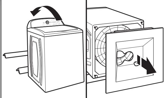
To avoid damaging floor and washer, place cardboard supports from shipping carton on floor behind washer. Use two or more people to tip washer back and place on cardboard supports. Remove shipping base.
