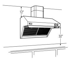
**8 ft. ceilings:** When the hood is installed 32" above the cooking surface and there is no soffit or upper cabinetry, order one 12" and one 6" duct cover accessory.
