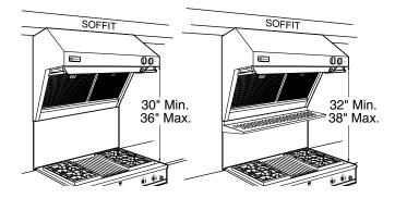
In this installation the ductwork running from the top of the hood will be concealed in the soffit or upper cabinetry.
