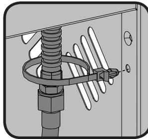
Clip hose to side panel using hose retainer clip supplied.
