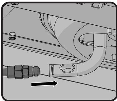
Fit orifice into burner tube and secure with hose retainer clip supplied. Attach the wire to the side burner electrode.
